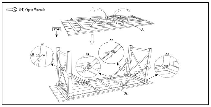
Lay down Table (A) on padded non-marring surface, lift legs upright to 90 degrees untill the braces are locked, as shown in the diagram. **Tighten 16 nuts on supporting brace using Open Wrench (H). DO NOT OVER TIGHTEN.**
